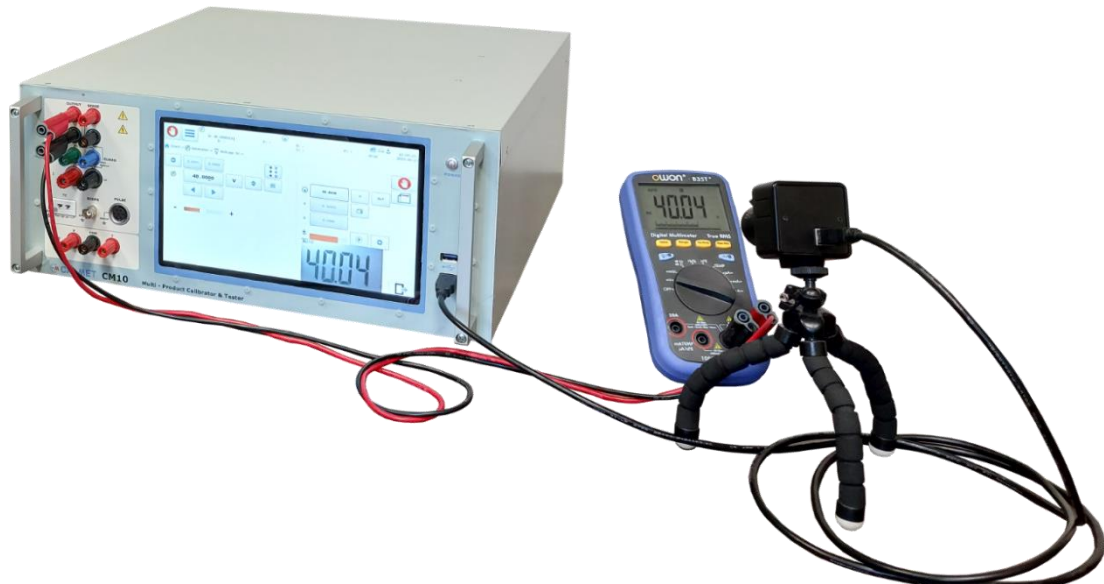
Automatic calibration of the 7-segment display DMM by using USB Camera
