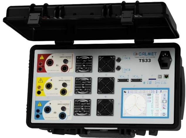
The Calmet TS33 portable test system consists of a three-phase reference meter of accuracy class 0.02% (or 0.04% or 0.1%) and an integrated three-phase current and voltage source up to 3x120A/600V. The TS33 is designed for analysis of complete metering installations and local mains conditions.
