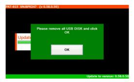
Remove USB flash disk and press **OK** to complete the upgrade procedure.
