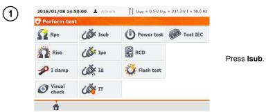
Before starting the measurement, similarly to the measurement of PE continuity test (see 4.2 of this manual), following parameters must be set: **test duration, limit**.
