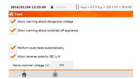
If each test is meant to be executed one after another automatically Perform auto-tests automatically option must be selected. Otherwise each test will be executed separately by pressing START button.
