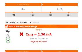
Negative test result: I<sub>SUB</sub> > LIMIT
