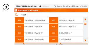
Select the test number from the list or scan the code from the proper barcode (or 2D code) with the barcode reader (PAT automatically detects connected barcode reader). If the test method was previously assigned to the selected appliance, it will now be highlited.
