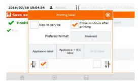
When selecting **Perform auto-tests automatically** in the menu (see sec. 3.3.5), the label is printed immediately after pressing (Save).
