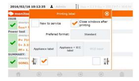
When **Printing Label** window shows up, select **New to service** if the device is being tested for the first time, and if using reference strikes also tick the approriate box, corresponding to the selected retest period (see 3.3.5).
