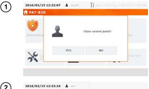
To change user, the current one has to log out. Press his name on the top of the screen in the main menu and then press**YES** to confirm.
