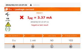
Negative test result: I<sub>PE</sub> > LIMIT
