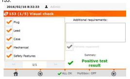
Perform visual inspection of the appliance and mark proper checkboxes if the inspection result was positive. If every-
