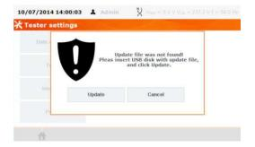
This screen shows up only when USB flash drive is not inserted or it's not detected/proper. Insert USB flash disk with upgrade files on it and press **Update** to upgrade the firmware or press **Cancel** to cancel upgrading procedure.
