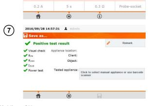
Upon completion of the measurement procedure a summary screen is displayed. The results can be saved into memory (see section 5).
