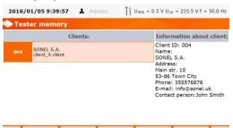
To add new object or appliance press client's name and press (Open) or double-press client's or object's name to add subobject within the selected object.
