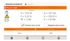
Upon completing the test read the results and compare them with the technical data of the tested device. The assessment of the correctness of the test results can be performed by selecting the proper field in 'Positive test result' or 'Negative test result'. When saving test results in the memory, this assessment will also be saled along with the results.
